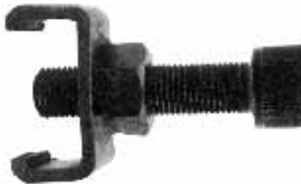
Prestons XL Tappet Guide Puller Removes press-fit tappet guides from the crankcase after tappet body adjusting screw is removed. 2098
