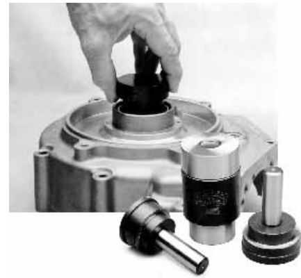
Jims Timken Bearing Race Installer Use to press a race in straight in the left side crankcase on BT 1969-99 and XL 1977-on models. For 1969-on Big Twin use Jims tool #31459. 31558
