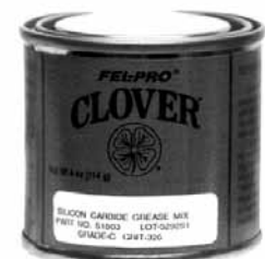
Clover Oil Based Lapping Compound 16 Oz. can. Use on valves for a good seal and with all Jims lapping tools. Available in 2 grits- 1 for roughing-in and 1 for finish work. 31591 Coarse 220 grit (micron finish of 32) 31592 Fine 320 grit (micron finish of 16)
