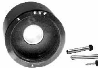
Sifton Cam Gear Tool to 1999 Tool makes it easy to time and install cam gears for the quietest possible cam gear train. +/- 4-8 degree timing as well as 0 degree for stock. Include alignment-press fixture, cam gear degree index pins, camshaft index pins for most makes of cams and instructions. Fits pre-Evo. 26150
